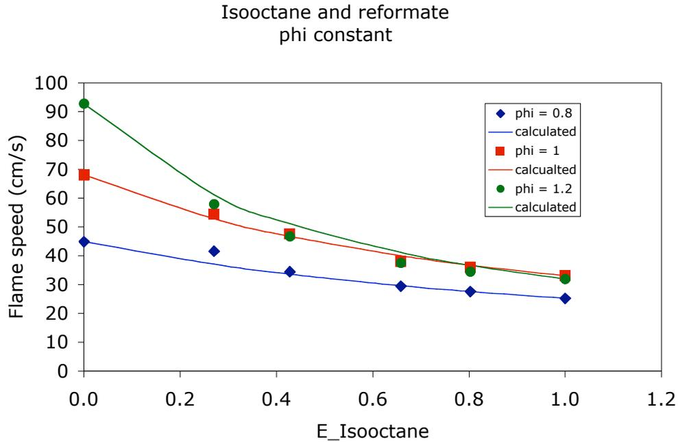
Figure 4. Interpolated experimental values of flame speed (from results of Huang [18]) of isooctane-reformate gas mixtures, for constant values of  $\phi_{\text{exhaust}}$  as a function of the isooctane energy fraction; also plotted is  $v_{\text{mixture}}$  (solid curves) using eq (1).
