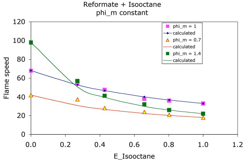
Figure 3. Experimental flame speed of isooctane-reformate mixtures as a function of the fraction of the isooctane energy fraction, for constant values of  $\phi_m$ . (points using experimental data of Huang [18]); also plotted is  $v_{mixture}$  (solid curves) using eq (1).
